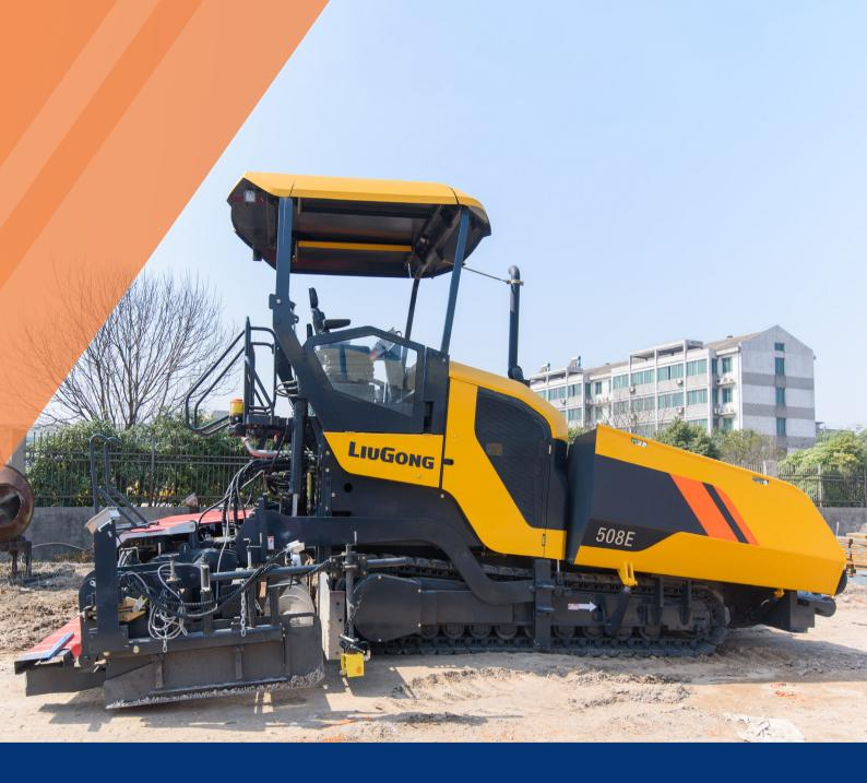
EngineCummins QSB5.9-C210Rated Power152 kW (204 hp / 207 ps) @ 2,000 rpmBasic Paving Width2.5-4.5 mMaximum Paving Width6 mMaximum Paving Thickness350 mmOperating Weight20,000~23,000 kg
