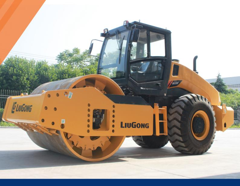
EngineShangchai SC9DK240G3Rated Power177 kW (237 hp / 241 ps) @ 2,200 rpmNominal Amplitude Range2.1 / 1.2 mmVibration Frequency Range28 / 32 HzCentrifugal Force Range520 / 400 kNWorking Width2,200 mmOperating Mass30,000 kg
